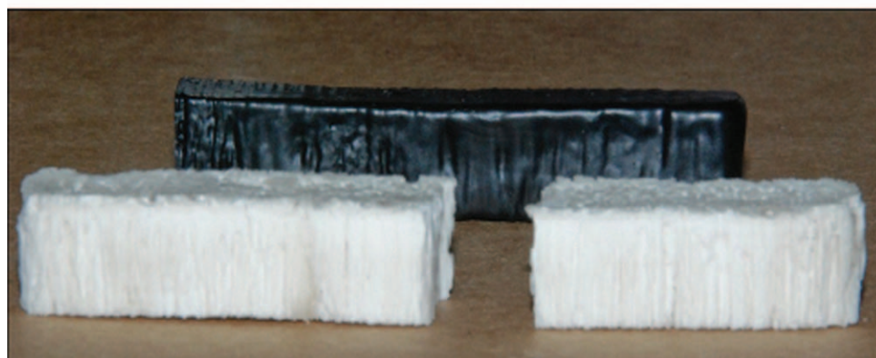
Figure 6 Comparison of the mechanical behavior before and after coating (top) with an image of complete failure without coating (bottom). [Color figure can be viewed in the online issue, which is available at wileyonlinelibrary.com .]
